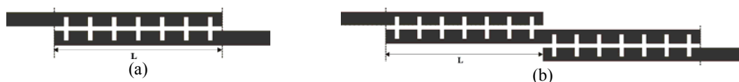
Fig. 5 Layouts of one stage PNCML section and filter, w=0.6\text{mm} , s=0.2\text{mm} , L=7.0\text{mm} , T=1.0\text{mm} , t=0.2\text{mm} .
