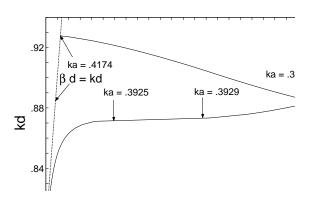
Figure 2:  $kd - \beta d$  diagram for traveling wave Figure 4: Lowest branch of  $kd - \beta d$  diagram of on array of spheres,  $\epsilon_{\rm r}=10,\,\mu_{\rm r}=1,\,ka=1.1.$
