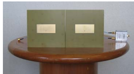
Fig. 2. Photo of the differentially-driven and single-ended microstrip antennas.
