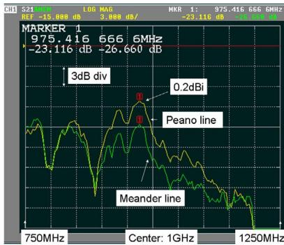
Fig. 7 Gain characteristics of meander and Peano line antenna
