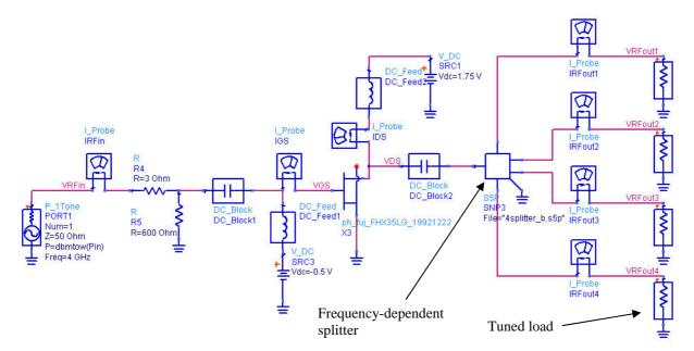
Fig. 3: Harmonic tuning simulation.
