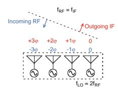
Fig. 2: Phase-conjugating array based on self oscillating mixers [4].
