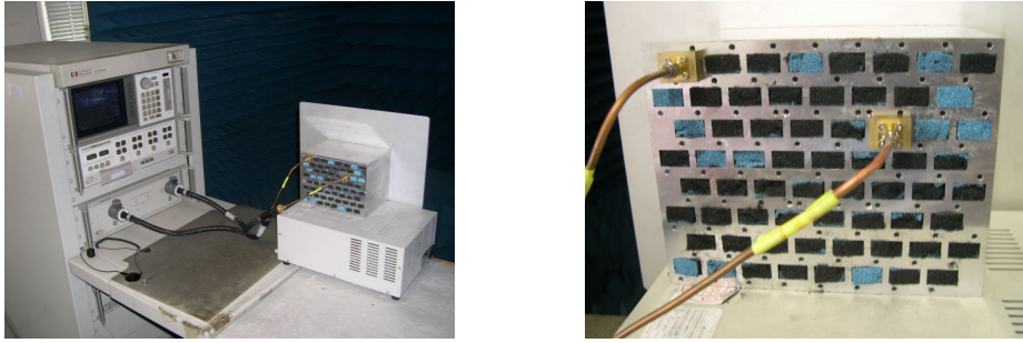
Figure 4: Fabricated 8 \times 8 subarray and its S-parameter measurement setup.
