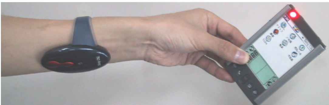
Fig. 1 Transmission system using the human body as a transmission channel [2].
