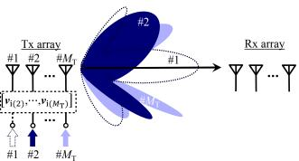
Fig. 1. Conceptual sketch of the proposed self-interference reduction technique: weighted Tx array nulls a direction to Rx array with a cost of one MIMO stream.
