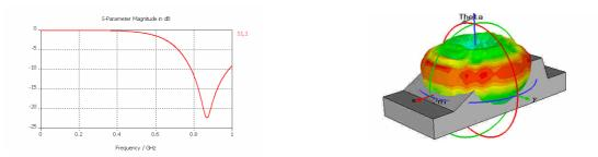
Figure 3: Simulated S<sub>11</sub> and 3-D farfield radiation pattern of the whole structure in CST.
