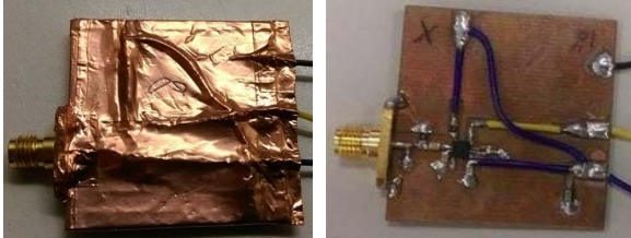
Fig. 2. Fabricated RF power detecting modules (LT5538) with and without copper foil shielding.
