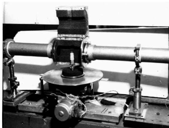
Fig.2. Measurement cell in the MCR made on the base of the circular ribbed HDB with D = 40\text{mm} .
