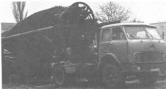
Fig.5 Construction of ground mobile antenna of 12m diameter in setting and functional view
