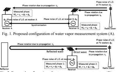
Fig. 2. Proposed configuration of water vapor measurement system (B).
