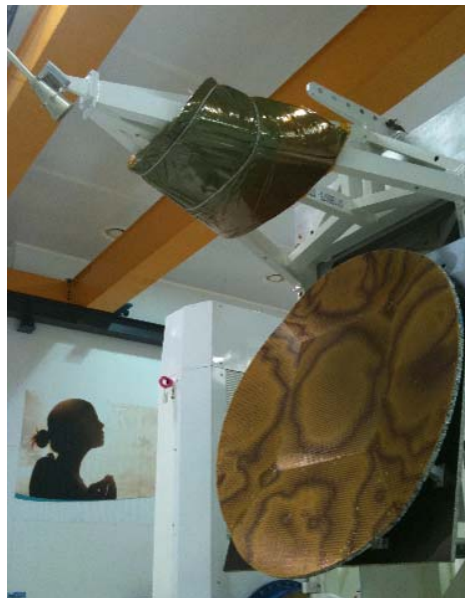
Figure 1: The 1.3 m faceted reflectarray breadboard
