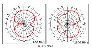
Fig. 5: Measured radiation patterns at 900 MHz and 1800 MHz for the antenna shown in Fig. 4.
