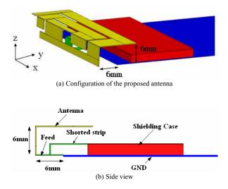
Fig. 1: Geometry of the proposed high integration GSM/DCS antenna in a mobile phone.
