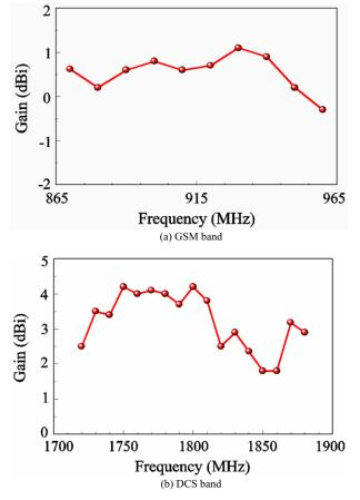
Fig. 6: Measured antenna gain of the proposed antenna.
