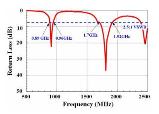
Fig. 4: Measured return loss of the antenna shown in Fig. 3.
