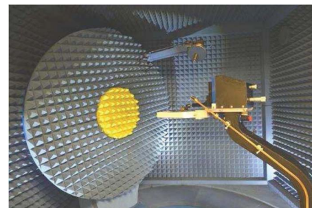
Fig 2. Orbit/FR \mu Lab on-chip measurement setup.
