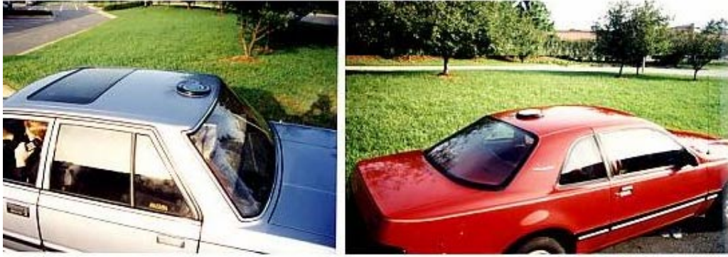
Figure 1. Multifunction SMM antennas mounted on rear rooftop of two passenger cars.
