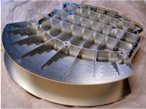
Fig. 3. Fabricated lens beamformer in Ku band producing six beams (Ports are numbered from 1 to 6, starting from the right side)
