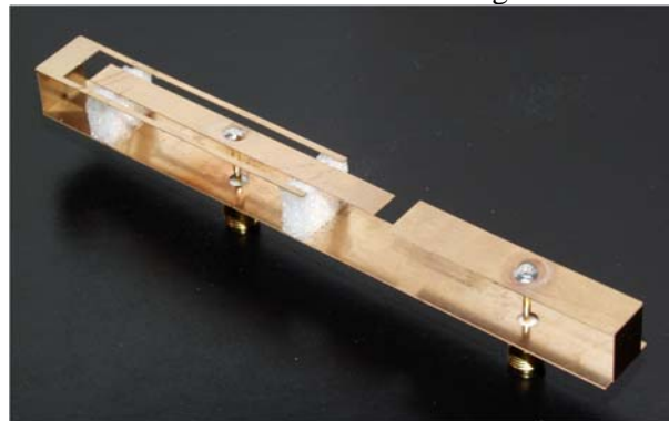
Figure 4 : double PIFA for GSM/DCS (feed point to the left) and UMTS bands
