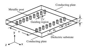
Fig. 1. Schematic of a post-wall waveguide.
