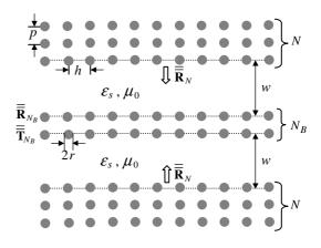
Fig. 3. Two-parallel post-wall waveguides "a" and "b" coupled through  $N_B$  -layered post-wall barrier.
