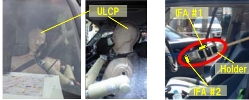
Figures 4: Installation of MIMO antenna for MT.
