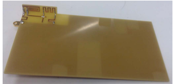
Fig. 2. Fabricated quad band GNSS reception antenna
