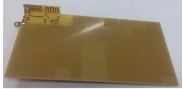
Fig. 2. Fabricated quad band GNSS reception antenna
