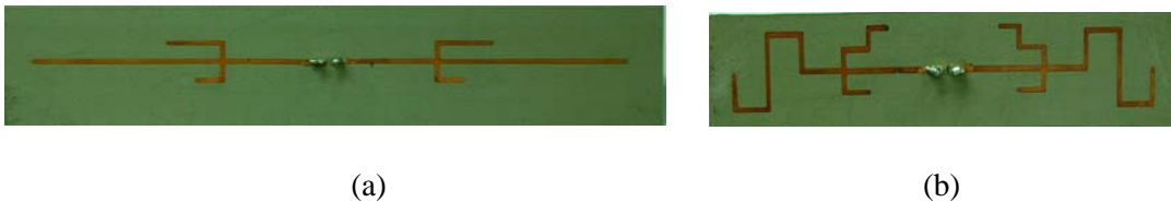
Figure 1: The Fabricated Multi-band Dipole Antennas: (a) Straight and (b) Meandered
