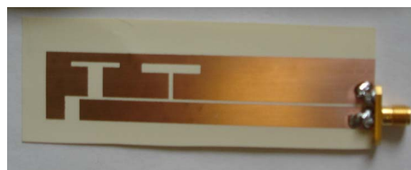
Re-designed LCP antenna
