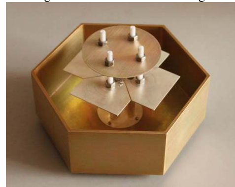
Figure 4. Photograph of the hexagonal cavity-backed dipole
