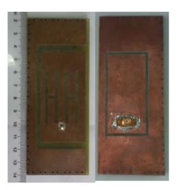
Fig. 8. Photo of the fabricated antenna.
