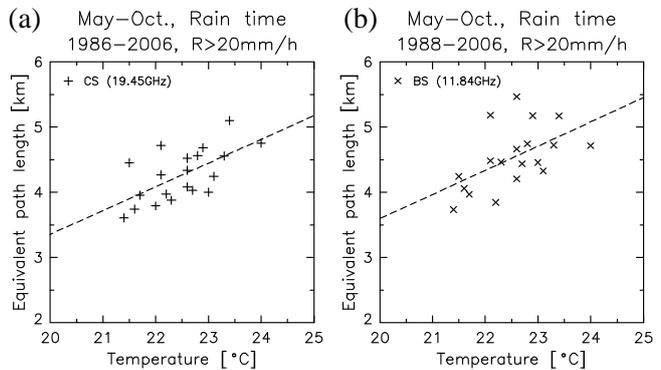
Figure 10: Scatter plot of yearly equivalent path length against ground temperature in rain time.
