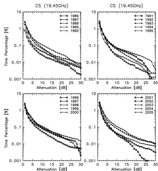
Figure 2: Cumulative time percentages of Ka-band rain attenuation obtained for 1986-2006.
