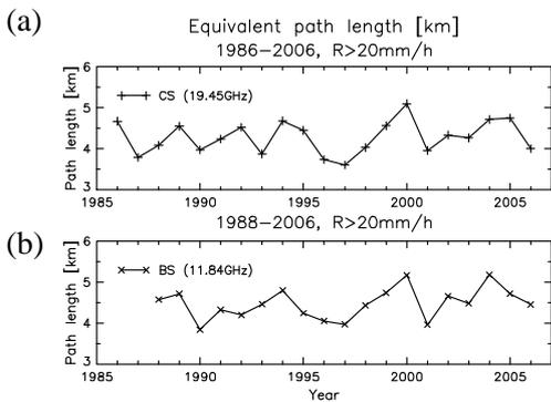
Figure 9: Equivalent path length for (a) Ka and (b) Ku band attenuation in each year.
