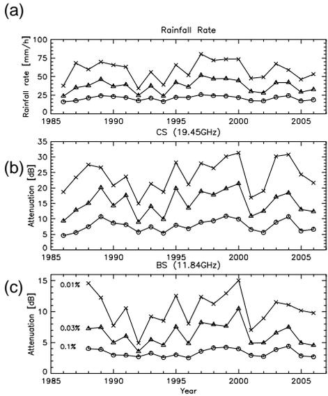
Figure 3: Equi-probability values of (a) rainfall rate, (b) Ka band, and (c) Ku band rain attenuation in each year.
