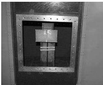
Fig. 10. Large open window of the metal enclosure, and showing the horn antenna inside the enclosure
