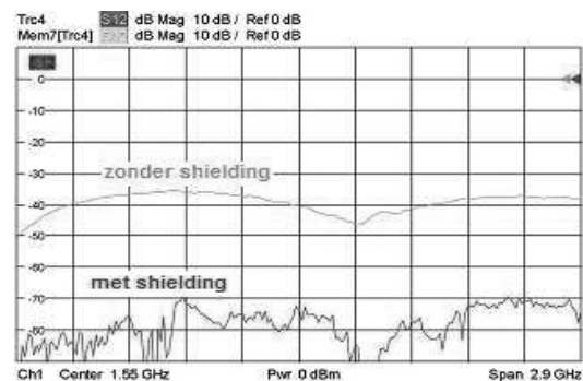
Fig. 8. Measurement of the induced signal in the stripline: upper trace for the naked microstrip (no CAN) and lower trace for the shielded microstrip
