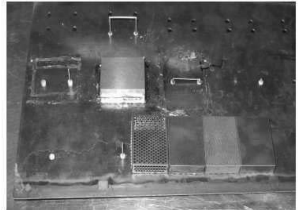
Fig. 2. Loop source and monopoles, with enclosures
