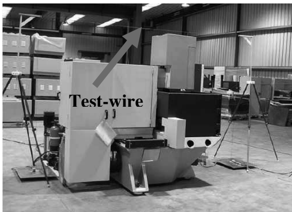
Figure 11. Sketch of the measuring setup for radiated emission using the test-wire method
