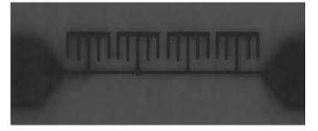
Fig. 6 Realized Filter with four PBG cells employing T-type microstrip  $line(4.4 \times 0.73 mm^2)$ .
