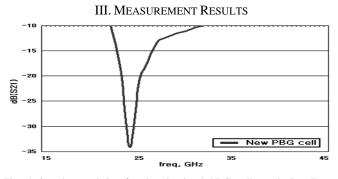
Fig. 4  $S_{\rm 21}$  characteristics for the simulated PBG cell employing T-type microstrip line.
