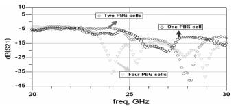
Fig. 9 Dependency of Band rejection characteristics on the number of cells.
