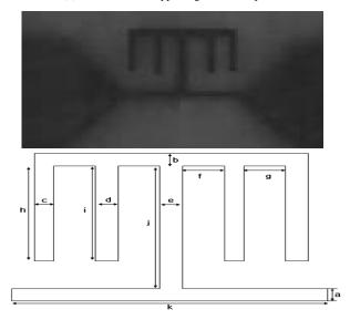
Fig. 3. The proposed microstrip PBG cell employing T-type microstrip line  $(1.1 \times 0.73 \text{ mm}^2)$ .
