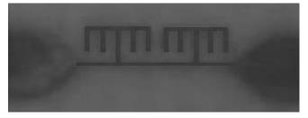
Fig. 5 Realized Filter with two PBG cells employing T-type microstrip  $line(2.2 \times 0.73 mm^2)$ .
