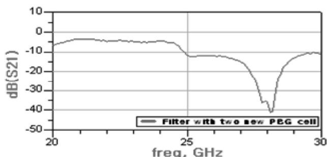
Fig. 7 S_{21} characteristics for the realized filter with two PBG cells employing T-type microstrip line.
