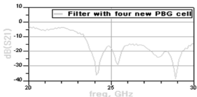
Fig. 8 S_{21} characteristics for the realized filter with four PBG cells employing T-type microstrip line.
