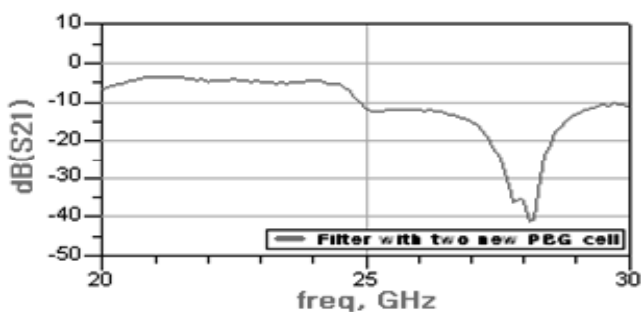
Fig. 7 S_{21} characteristics for the realized filter with two PBG cells employing T-type microstrip line.
