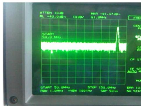
Fig.7 Result of the receiving signal from Helix Antenna with Plasma Antenna in Spectrum Analyzer.
