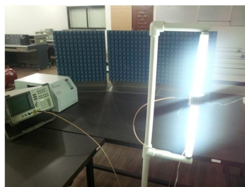
Fig.6. Connection of the antenna and Spectrum Analyzer before the test
