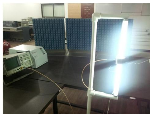
Fig.6. Connection of the antenna and Spectrum Analyzer before the test
