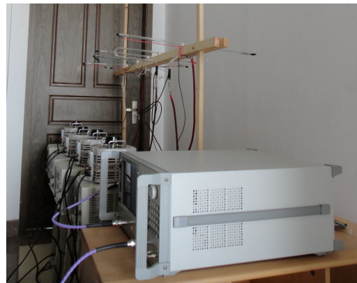
Figure 7 Plasma Yagi antenna measurement layout
