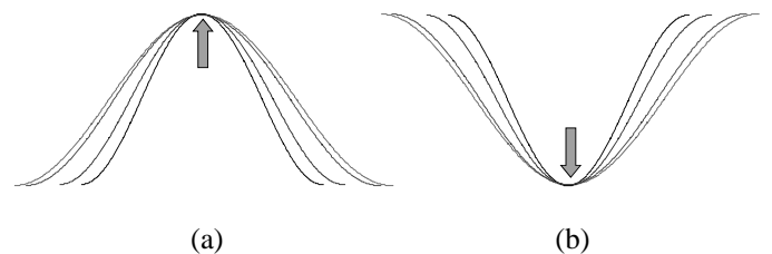
Fig. 5 Two worst conditions of coupled noise to bring the largest timing variation. Two noise waveforms with high-positive peak (a) and with low-negative peak (b)
