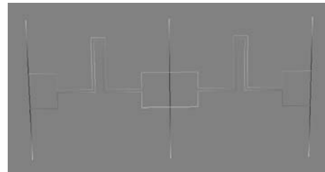
Fig.6 Current distribution on the PDAA using the odd mode meander line
