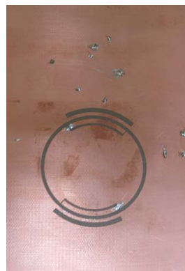
Fig 5: Fabricated Reconfigurable Active Antenna
