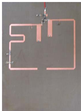
Fig 5: Fabricated Reconfigurable Active Antenna
