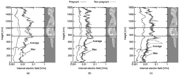
Fig.4 Distributions of maximum and averaged value of the induced electric field along the height. The area between thick dashed lines is the existing region of the amniotic fluid for the pregnant-woman model. Incident magnetic field directions are (a) TOP, (b) LAT, and (c) AP.
