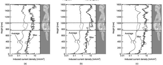
Fig.2 Distributions of maximum and averaged value of the induced current density along the height. The area between thick dashed lines is the existing region of the amniotic fluid for the pregnant-woman model. Incident magnetic field directions are (a) TOP, (b) LAT, and (c) AP.
