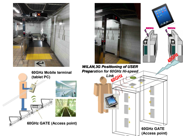
Fig. 6 Image of a Gigabit access transponder equipment at the escalator.
