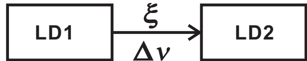
Fig. 1 Schematic setup of an optical injection system. The dynamics of the slave laser (LD2) can be controlled by varying the injection strength \xi and the detuning frequency \Delta\nu from the master laser (LD1).
