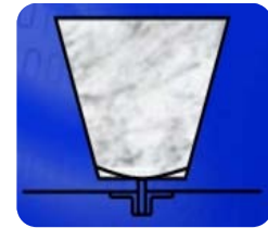
Figure 4: Trapezoidal Disc Antenna J. A. Evans and M.J. Ammann, 1999
