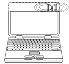
(b) Printed type mono pole Yagi-Uda antenna for beam-steering
