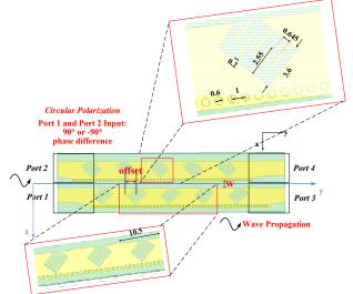
Fig. 1. Configuration of the reconfigurable antenna
