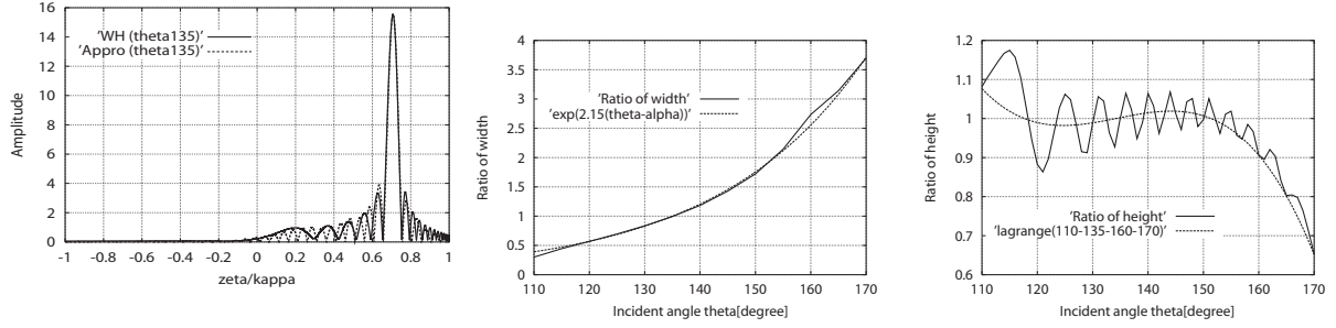
Figure 2: WH and approximate solutions ( f = 300\text{MHz} , \theta = 135^\circ , Figure 3: Width of main lobe W^w(\theta) . Figure 4: Height of main lobe W^h(\theta) . b = 10.1\lambda ).
