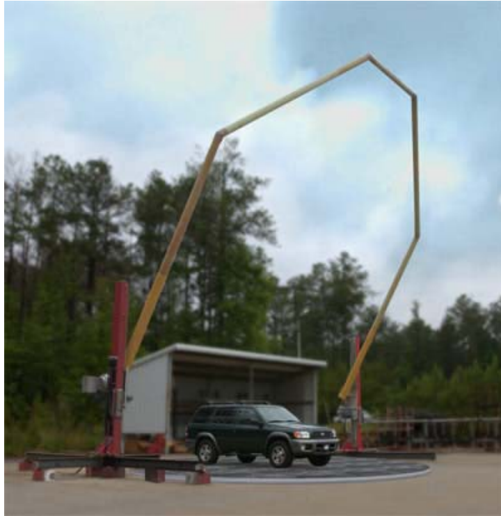
Figure 5. Spherical near-field telematics measurement system
