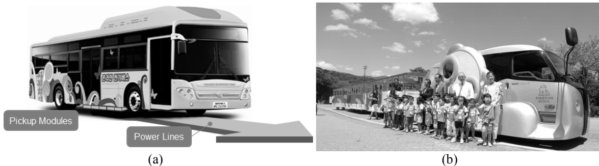
Figure 1: (a) The On-line Electric Vehicle (OLEV) and the power transfer system using power lines placed underneath the road surface for non-contact charging (b) An OLEV commercially used at Seoul Grand Park
