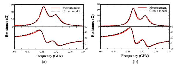
Fig. 2. Simulation using the circuit model and measurement (a) in the free space and (b) with the Wheeler cap.
