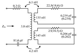
Fig. 1. Circuit modeling for the CP microstrip antenna
