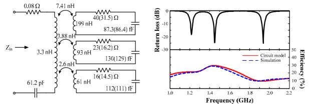
Fig. 4. Circuit modeling for triple-band antenna
