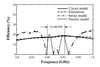
Fig. 3. Efficiency of the CP microstrip antenna
