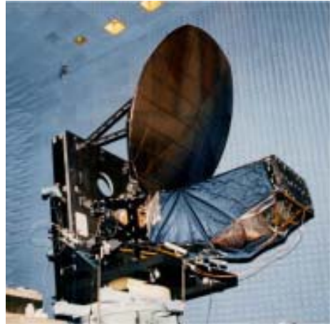
Fig. 9 N-STAR Ka-band Offset Gregorian Antenna
