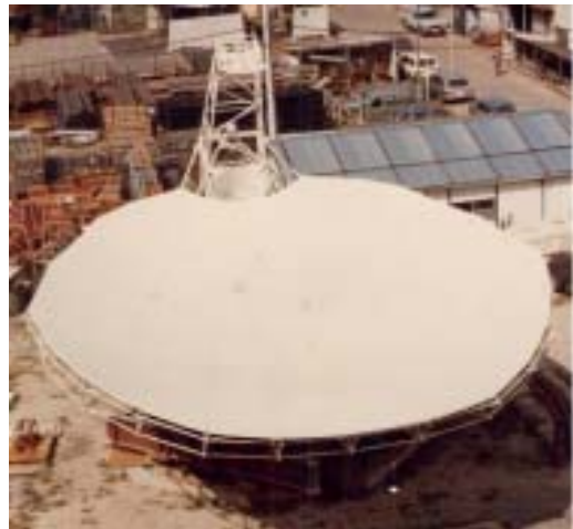
Fig.4 NTT 11.5m Ka-band Offset Cassegrain Antenna
