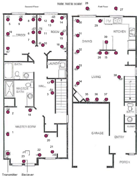
Fig. 1: Townhouse layout where channel impulses are measured. The spots in the figure denote the locations of transmitter and receiver antennas.
