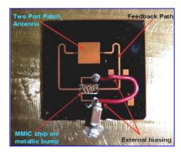
Fig.7 Final Antenna circuit with biasing circuit
