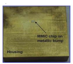
Fig. 6 MMIC amplifier chip on metallic bump
