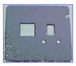
Fig. 5 Micromachined Active Antenna: (a) Design layout on silicon (b) Backside aligned cavity *Micromachined Active Antenna Element (on 270µm Silicon substrate)*
